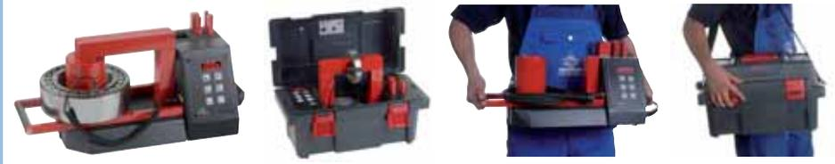
**WORKBENCH MODELS, swivel arm, 3.6 and 8 kVA, work pieces up to ± 350 kg**
