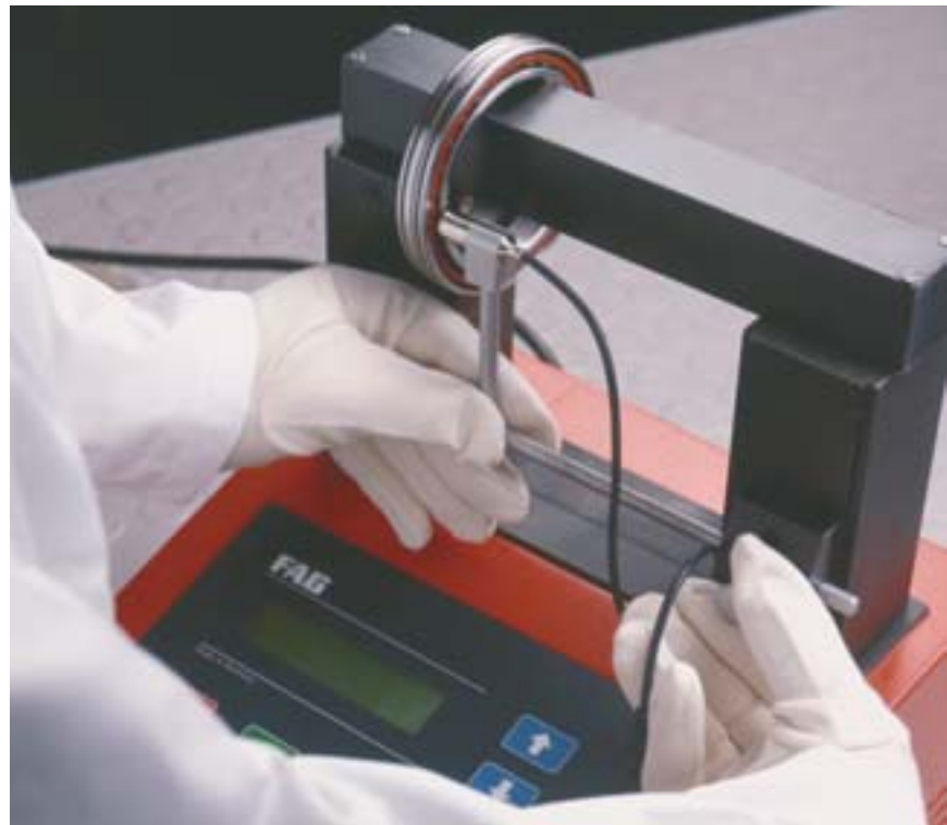
40: Heating of a precision bearing using induction heating device
